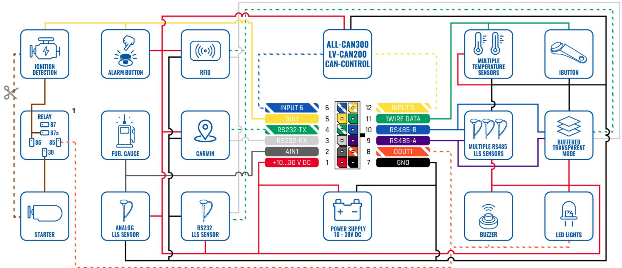
Figure 3 FMM125 Wiring scheme
