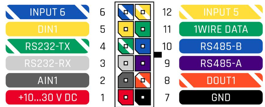
**Figure 2 FMM125 2x6 socket pinout**
